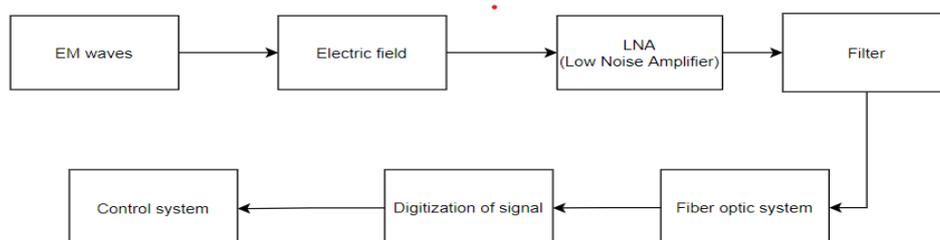
Fig. 1. Block diagram of signal reception and processing by an antenna
